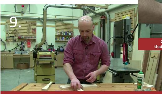
Cut along the pencil lines to make a spacer block that will locate the handle centered on the mallet head.
